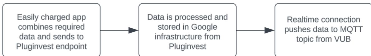
Figure 4: Real-time data connection between Easily Charged app (Jedlix), Pluginvest and the Vrije Universiteit Brussel
